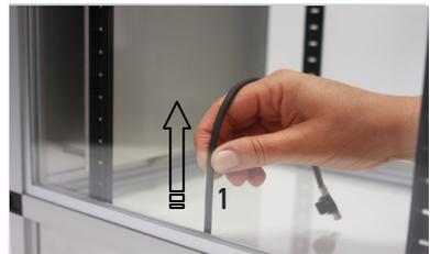
» Once the cable is long enough to reach the required position you can attach the temperature sensor (1) by clicking it into the suspension arrangement (2).
