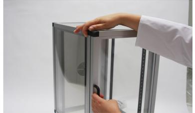
» **Please note:** Due to the strong magnetic lock, it is harder to open the door the longer it was closed before. This is normal and can be compensated by pulling stronger than in the everyday use.
