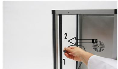
» Mount the rails (3) horizontally in pairs on both sides of the suspension arrangement (2). The engagement of the rail (3) is clearly audible. For a better orientation, the levels are marked by numbers on the suspension arrangement (2).
