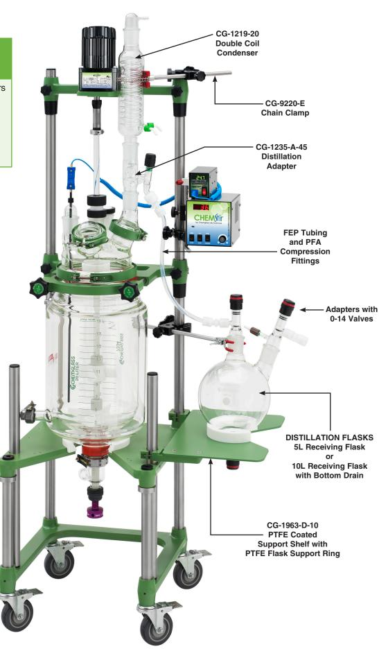
CG-1965-D DISTILLATION KIT FOR 10 and 20L PROCESS REACTOR SYSTEM
